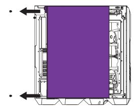
Remove screws from the left side of the glass panel. Then remove the glass panel.
