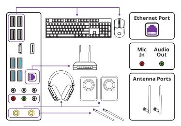
Connect your keyboard, mouse, audio and antennas/ethernet to their matching ports on the motherboard.
