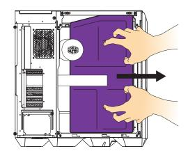
Carefully remove the protective foam inside the PC. Then put the glass panel and screws back on.
